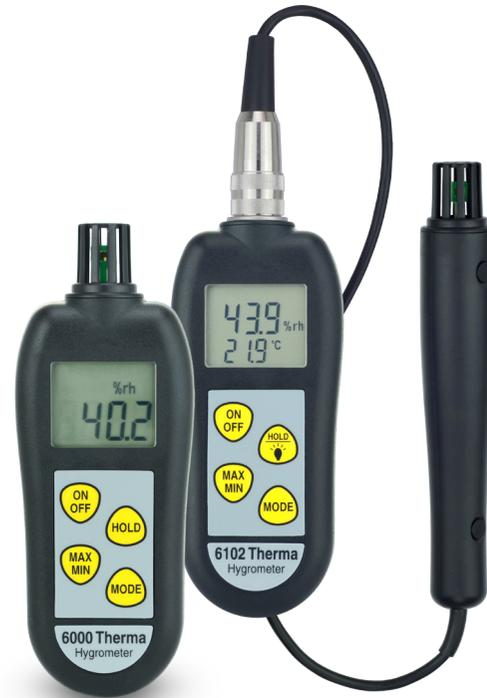
**INSTRUMENT OPERATION** - The instrument is switched on by pressing the ON/OFF button. To obtain accurate humidity measurements, allow the instrument to stabilise in the environment for a minimum of one minute. To maximise accuracy, allow airflow across the sensor.
