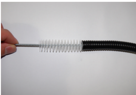
Fig. 67: Cleaning the pump hoses
