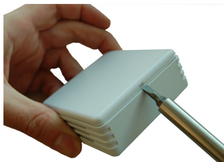
Fig. 11: Opening the cover
